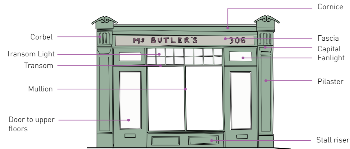
One example of a traditional shopfront layout
