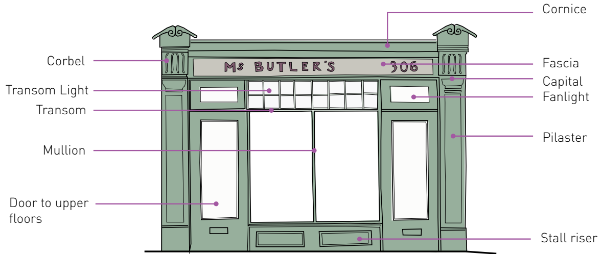
One example of a traditional shopfront layout
